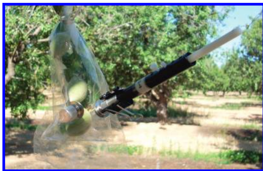
Figure 1. In situ VOC collection system showing the inert bag with enclosed almonds and SPME cartridge in place.
